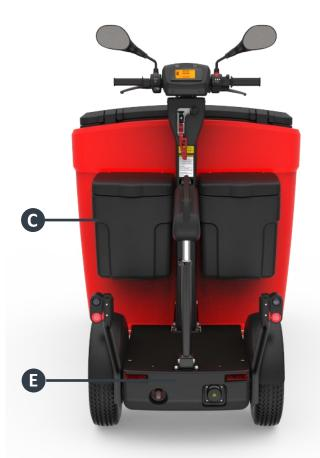
The front side of the loading compartment can be opened in order to facilitate easy loading and unloading of cargo.
